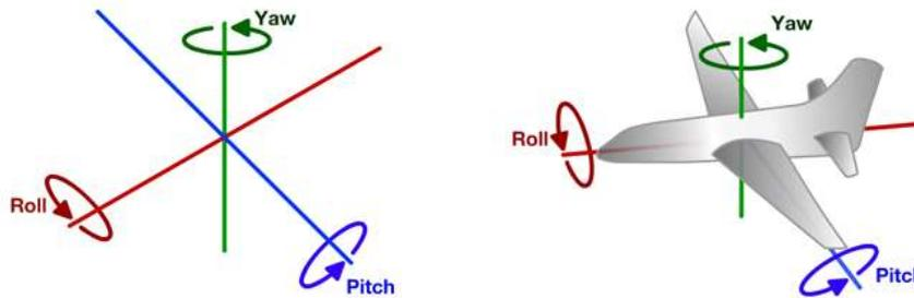
Fig. 2. Roll, Pitch and Yaw angles [14]
